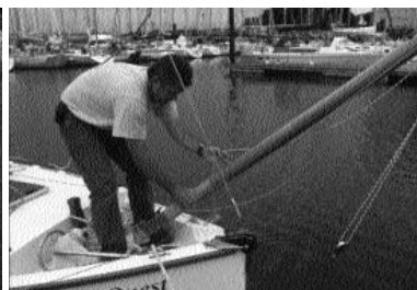
Lower it by taking up on the bobstay
