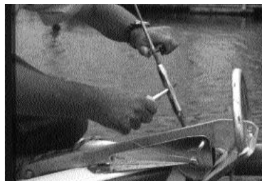
Fix the inner-forestay to hold the mast up
